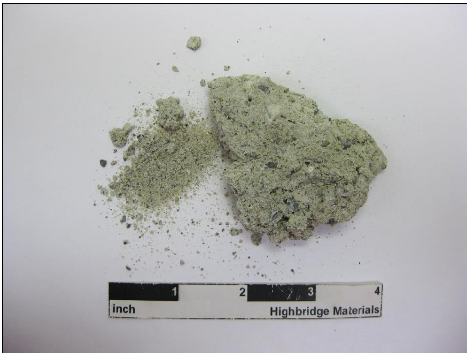
Figure 1: Photograph of the examined mortar sample provided to Highbridge for examination. The mortar has a uniform appearance with a light gray color. The cured product is cohesive, but the paste is moderately soft and highly permeable. There are also some hairline cracks visible in the sample piece.
